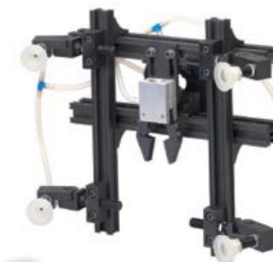
5. Finally, mount the nipples, fittings and tubes. The EOAT is ready for use.
