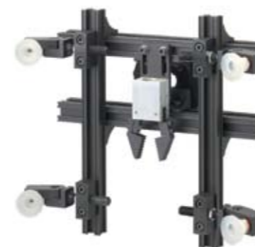
4. Now you can position the vacuum cups, gripping pliers and cylinders.
