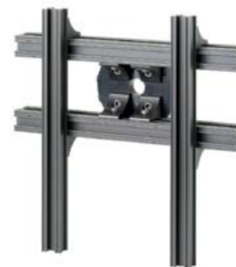
2. Mount the vertical profiles on the horizontal profiles. This gives you maximum flexibility in two directions for making adjustments for individual parts.
