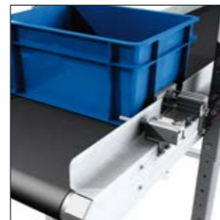
Stop cylinders and lateral positioning cylinders for boxes (optional).
