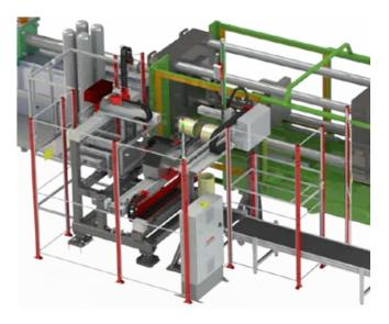
Modular concept for wrap around of large containers, with seperate stacking robot. Robotcell with two robots and one controller.
