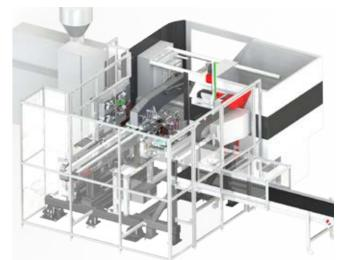
Modular concept for flat labels or wrap around, with quality inspection and seperate stacking robot. Robotcell with two robots and one controller.
